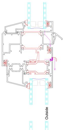
Machine 30mm x 5mm drainage slot 100mm from each end at minimum 300mm centres
