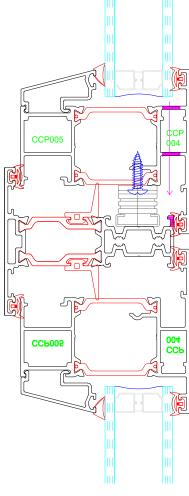
Machine 30mm x 5mm drainage slot 100mm from each end at minimum 300mm centres
